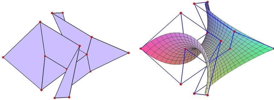
FIGURE 3. Enneper surface. Left: Control net. Right: Final surface.
